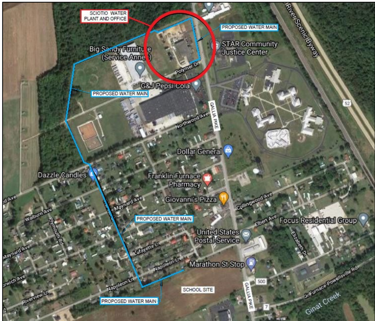
Figure 3. Proposed water main route (blue) and SWI water treatment plant and office (red)
